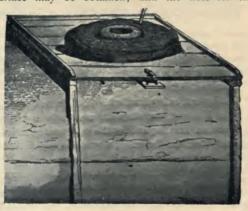
spindle, no longer a mere socket but a perforation passing entirely through the stone, is tightly fitted with a block of wood, also perforated, serving for a bearing for the spindle which passes through it and below the stone and rests on a narrow board beneath. The top stone, as usual, rests by means of its wooden rynd upon the top of the spindle. The adjustment for coarse or fine grinding is secured by raising or depressing the spindle (and so the top stone) from
